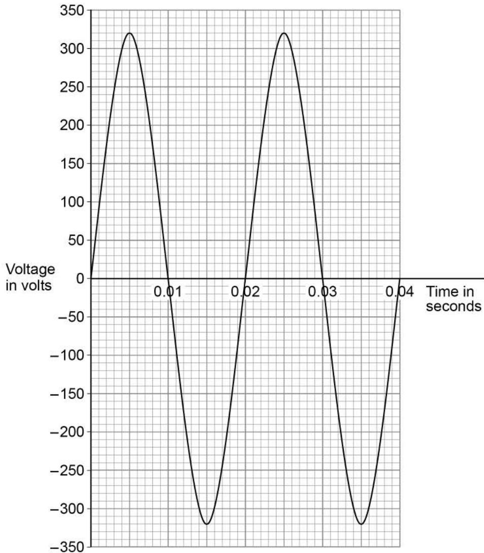
0 1 . 3 Use Figure 2 to determine the time period of the voltage supplied to consumers.
