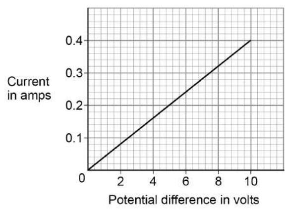
Determine the resistance of the resistor when there is a potential difference of 10 V across it.
