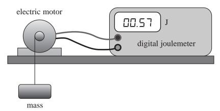
The students used a joulemeter to measure the energy supplied to the motor to lift a mass a distance of 75 cm. They repeated the experiment twice before increasing the mass.
