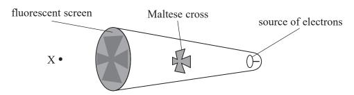
4 The electrons are produced by heating a metal filament.
