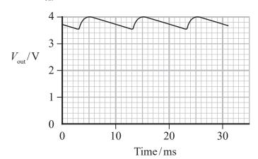
Determine a value for the capacitance of the capacitor.
