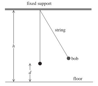
As the student was unable to measure the length of the pendulum directly, she measured the distance d from the bob to the floor.
