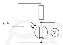
In daylight the voltmeter reads 3.0 V.
