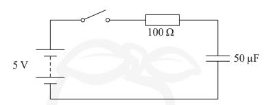
(a) Describe what happens to the potential difference across the resistor and the potential difference across the capacitor after the switch is closed.
