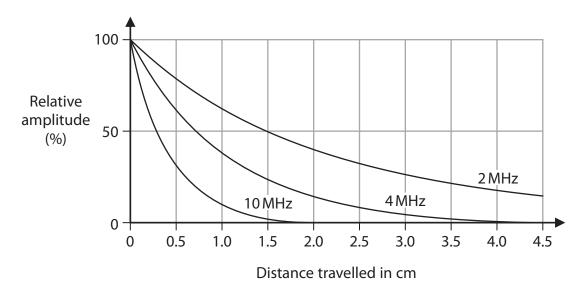
(i) Estimate the distance travelled by a 2 MHz wave when its amplitude is 25% of its original value.
