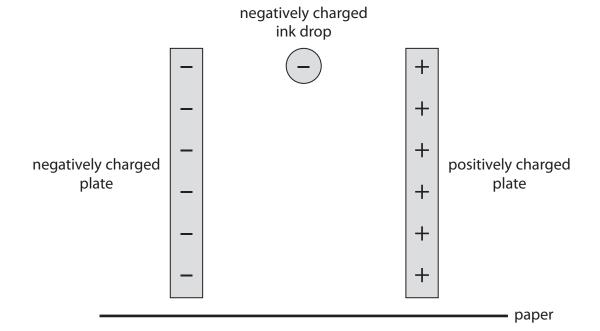
A negatively charged ink drop falls vertically between a pair of charged plates.
