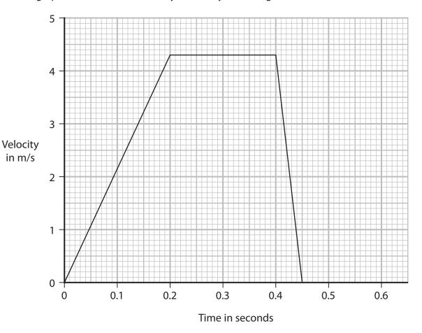
(a) Calculate the distance travelled by the car during the first 0.4 seconds.
