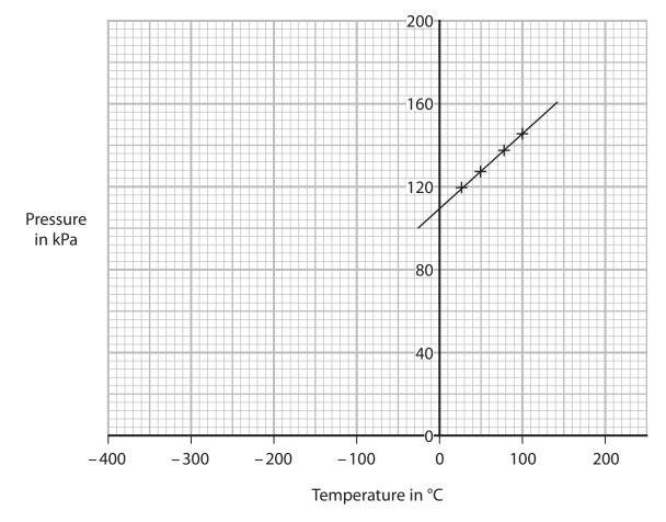
(i) Explain how these results show that there is a linear, but not proportional, relationship between the pressure of the gas and its temperature in °C.
