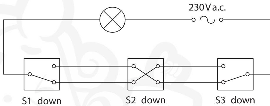
When all three switches are up, the lamp is on.
