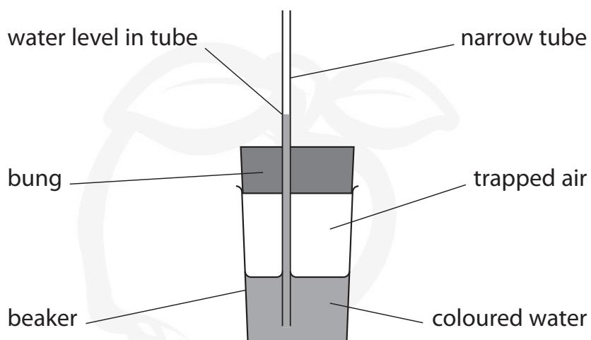
He uses a bung fitted with a narrow tube, and a beaker containing some coloured water.
