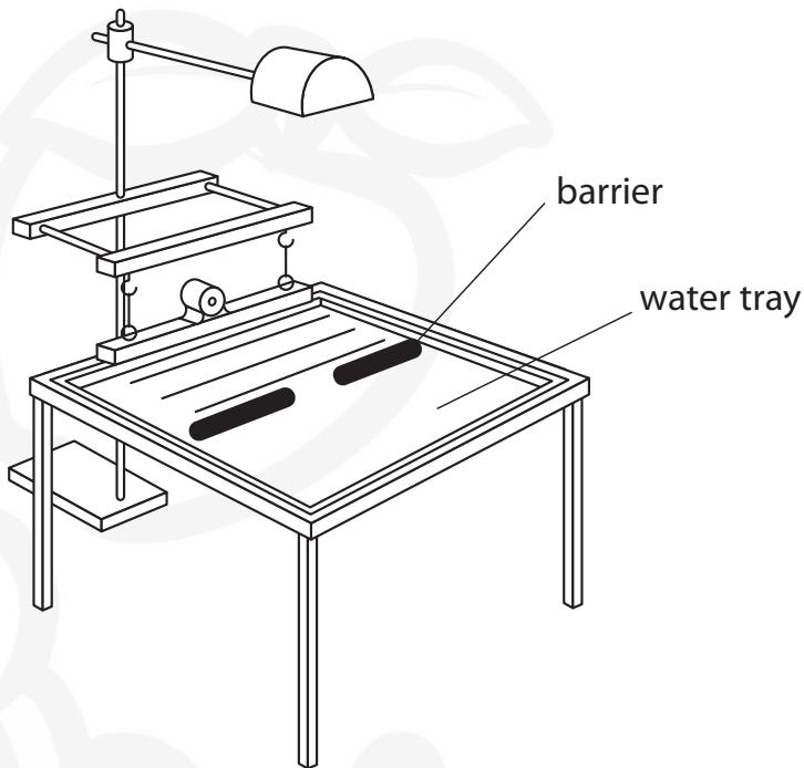
The ripple tank produces plane waves.
