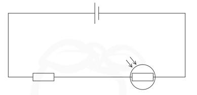
Explain why the power dissipated by the whole circuit changes as the intensity of the light incident on the LDR increases.
