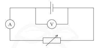
The student used the variable resistor to vary the reading on the ammeter. He recorded corresponding readings from the voltmeter.
