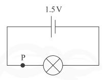
In 30 seconds, the charge passing point P is 0.4 C.
