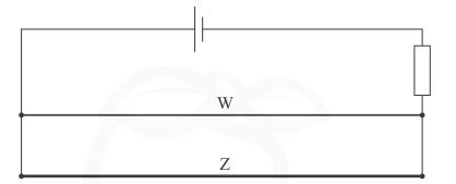
Wire Z has twice the diameter of wire W.
