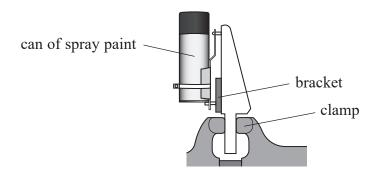
The bracket oscillates vertically with simple harmonic motion.
