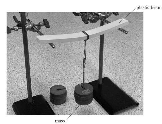
The beam bent downwards as shown.
