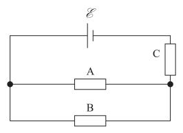
Describe how a single ammeter reading can be used to determine the internal resistance of the cell. You should add to the diagram to show the position of this ammeter.
