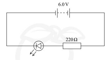
(a) When operating normally, the potential difference across the LED is 1.8 V.
