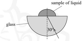
Determine whether this ray will be totally internally reflected from the boundary between the prism and the liquid.
