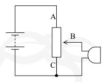
Explain how this circuit provides the variable output for the buzzer. The current drawn by the buzzer is negligible.
