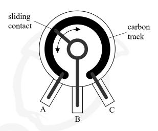
(a) The carbon track has a uniform rectangular cross-section.
