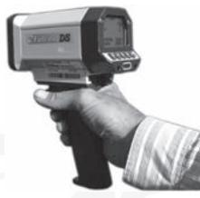
The speed gun emits pulses of infrared radiation every 0.250 s. The pulses are reflected by a moving car and then detected by the speed gun, which calculates and displays the speed of the car.
