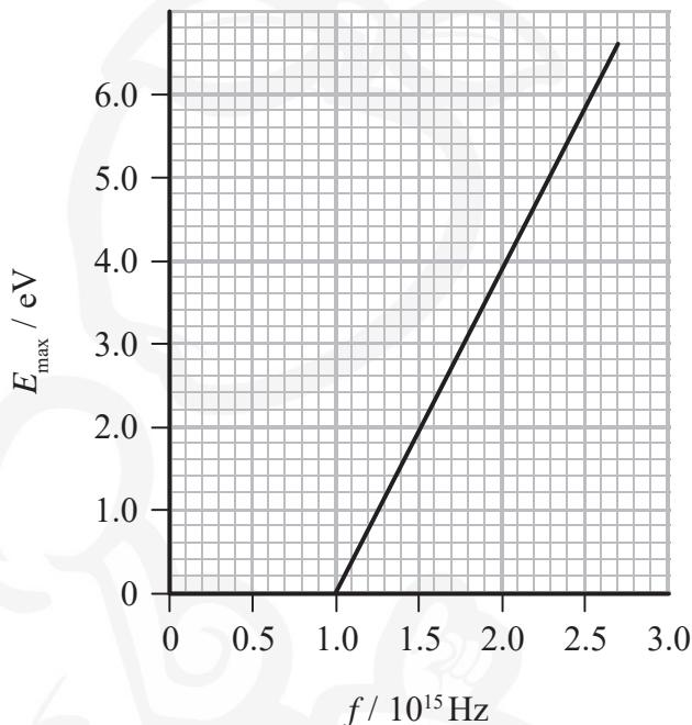
(a) The frequency at which the line crosses the  $x$ -axis is known as the threshold frequency.
