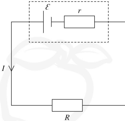
A cell has electromotive force  $\mathcal{E}$  and internal resistance  $r$ . It supplies a current  $I$  to an external circuit with resistance  $R$ .
