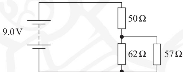
Calculate the total resistance of the circuit.
