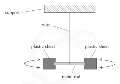
When the metal rod is rotated through an angle and released, the rod performs angular oscillations about a vertical axis through the wire. The plastic sheets dampen the oscillations as they move through the air.
