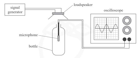
The signal generator was adjusted until a loud sound was heard at a particular frequency, known as the resonant frequency.
