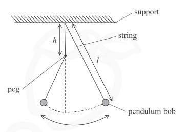
(a) Determine the time period T for the whole oscillation when h = 0.25 m.
