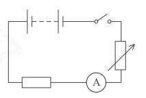
A student investigated whether the temperature rise of the water  $\Delta\theta$  was proportional to the current I in the resistor. For each value of current, the student refilled the beaker with water at the same initial temperature.
