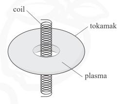
The plasma in the tokamak acts as a single conducting loop around the central coil.
