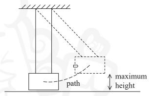
The pellet stays in the block of wood. The block of wood and pellet together then move along the path shown. The maximum height reached is measured.
