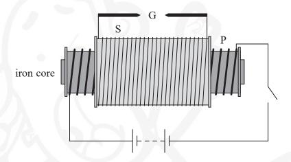
A coil of wire P is wound around an iron core. A second coil S is wound around P. The ends of S are connected to two thin metal rods with a gap G between them, known as the spark gap.
