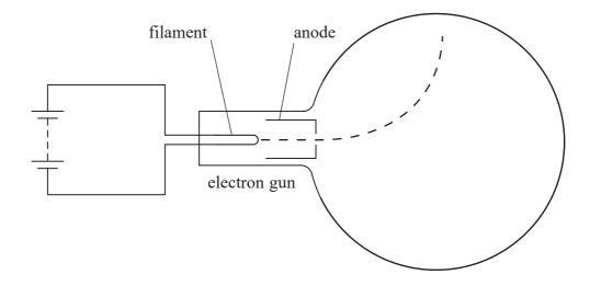
Electrons are released by a filament and accelerated towards the anode, producing a beam. A magnetic field is applied, deflecting the beam as shown.
