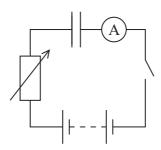
The capacitor is initially uncharged. When the switch is closed, there is a current in the circuit and the capacitor charges.
