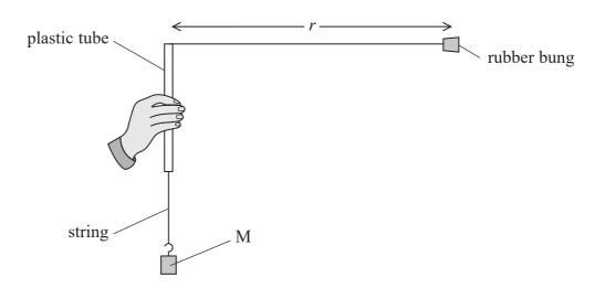
A small movement of the hand causes the rubber bung on the end of the string to move in a circular path of radius r. The rubber bung and the string may be assumed to rotate in a horizontal plane.
