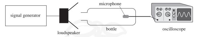
The frequency f of the sound produced by the loudspeaker is varied using the signal generator. The sound detected by the microphone is displayed as a potential difference V on the oscilloscope.
