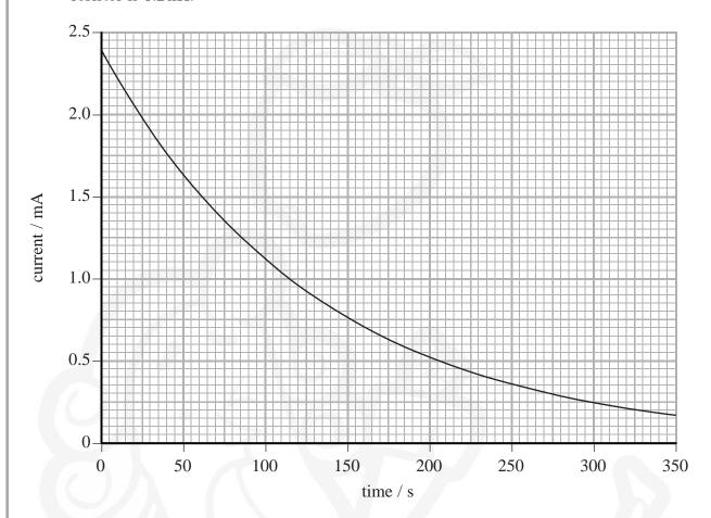
(i) Show that the capacitance of the capacitor is about 0.02 F.
