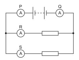
Which two ammeters read the largest current?
