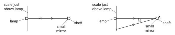
The beam from the lamp reflects from the mirror to give a small spot of light on a scale placed just above the lamp. The shaft and mirror rotate through 1°. The spot of light moves along the scale.
